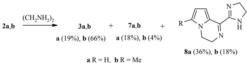
It was of interest to decrease the yield of compounds **3a,b** relative to compounds **7** and **8**. When the synthesis was carried out without solvent in a sealed ampul (140°C) with a ratio of starting compounds **2a,b** to ethylene diamine of 1:1.5 the desired result was achieved. The yields of compounds **3a**, **7a**, and **8a** were 10, 24, and 19% and for the methyl-substituted compounds 30, 21, and 24% respectively.
